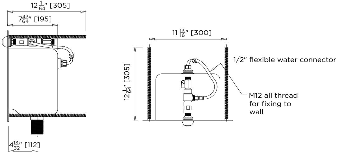
MODEL US-SRB Side Elevation and Plan
