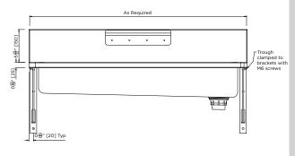
Troughs over 2000mm long are supplied with a centre support bracket
