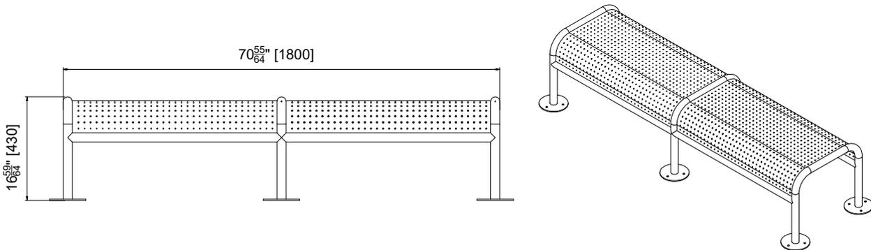
MODEL US-SF-B Front Elevation & Isometric View
