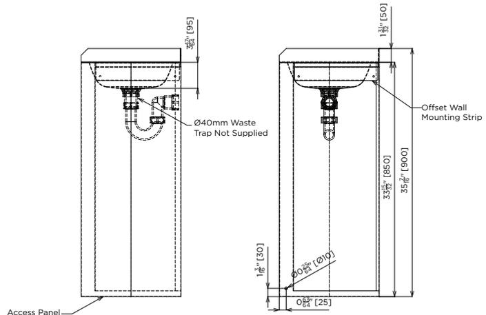
MODEL US-HBVRC-F Front and Side Elevation
