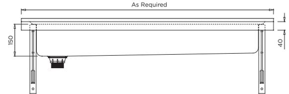
Troughs over 2000mm long are supplied with a centre support bracket
