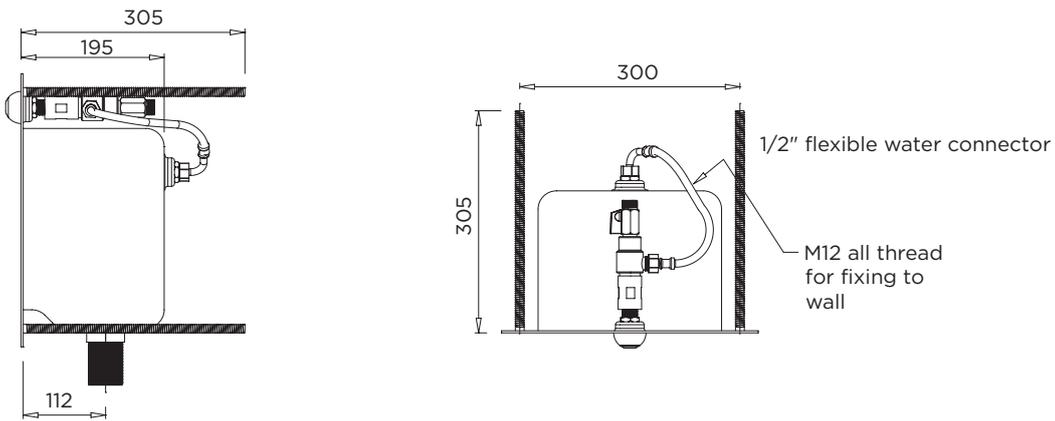
MODEL SRB Side Elevation and Plan
